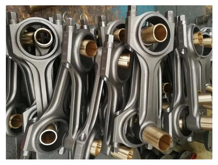
Hurricane Volvo 850 T5 C70 V70 2.3L 4340 Forged Steel X-Beam Connecting Rods 139.5mm are ready for install bushings.
