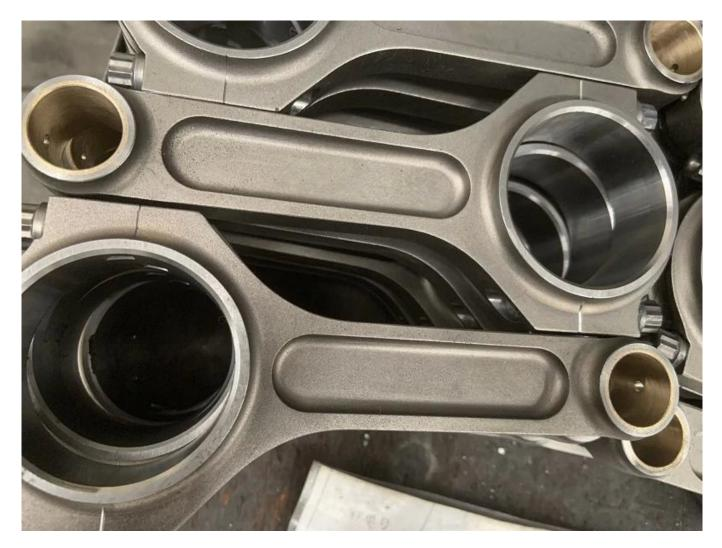
Our Volvo C70 MK1 2.3L B5234 T3 I5 139.5mm I beam Connecting Rod is ready for cleaning and packing.
