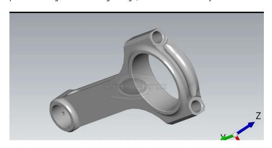
Per rod used H-beam design which increases twisting strength and rod reliability, also can save some weight and make the rods become more lighter. What's more, per rod's top of small ends finished with a small oil hole to make the oil can drip during the piston's compressing cycle, then to provide additional lubrication and cooling to the bushing in small end, which is good to secure the rods become more stronger and durable.
