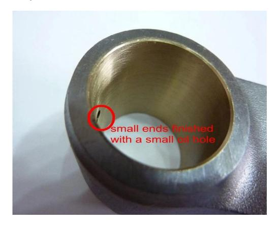
Per rod magnaflux inspected to ensure extreme reliability, and shot peened to improve fatigue life, honed with SUNNEN honing machine for superior tolerances to meet high quality standard.
