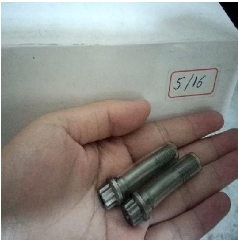
Note: hurricane 3/8 race spec connecting rod bolts.
