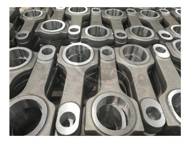
2). Designed with <u>I-beam shape</u> for optimum reliability in the racing industry
