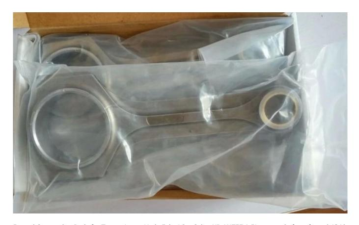
Forged Connecting Rods for Toyota Lexus Yaris Echo Vios Scion XB 1NZFE 1.5L are made from forged 4340 chrome moly steel, heat treated to increase tensile strength and are shot peened to increase fatigue life. Toyota 1.5L VVT-I 1NZ 1NZ-FXE 1NZ-FE Connecting Rods have a wear resistant bronze bushing for long wrist pin life and feature <a href="https://example.com/hurricane-3/8 fasteners">Hurricane-3/8 fasteners</a>.
