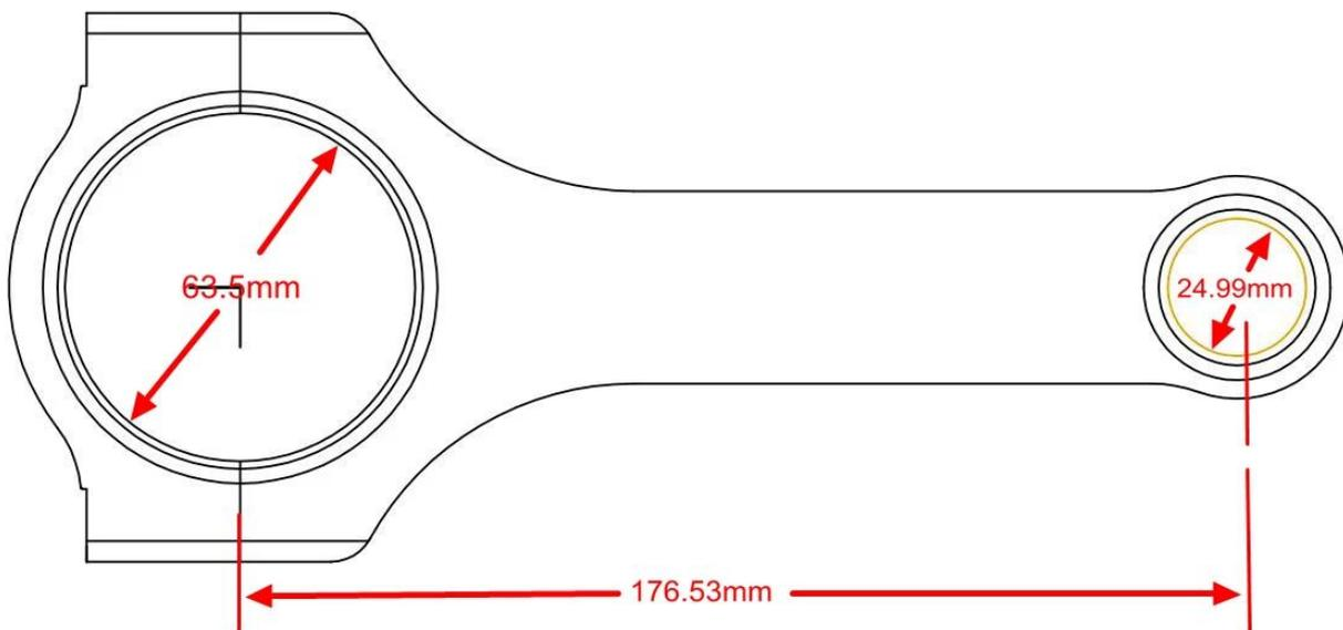
Those rods for 6.4L Chrysler. Hurricane connecting rods are honed, pre clearance and weight balanced, (+/-1g each set), which means less time in a machine shop, and you can use/sell them when rods in hand. For more chrysler connecting rod, please [click here](#), if you have any question or inquiry, Please [fill out this form](#) and we will get in touch with you shortly.
