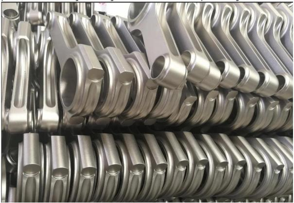
Finally, package with weight tolerance less than +/-1g in one set, which 8 pieces per set.
