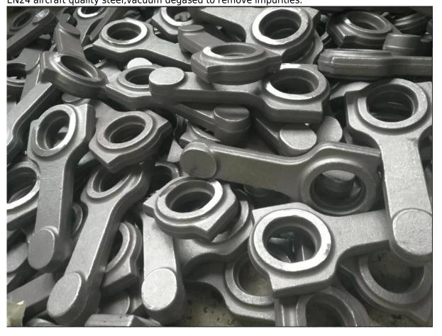
All surfaces are shot blasted and micropolished before finishing machining. It it relieve stress and improved fatigue life.
