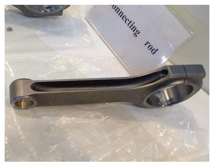
These 6.350" turbo Buick V6 connecting rods are heat treated and shot peened for added strength. Those considering a long rod for the 3.8L or 4.1L engine will surely appreciate the craftsmanship that goes into these h-beam steel connecting rods. They will perfectly match your 1986 or 1987 Buick Grand National, T Type, Turbo T, or GNX 3.8 liter turbo V6 engines.
