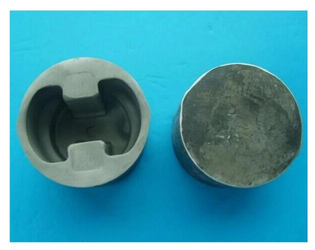
Although The piston inner side is forging surface not finish machining, we still make it very smooth.
