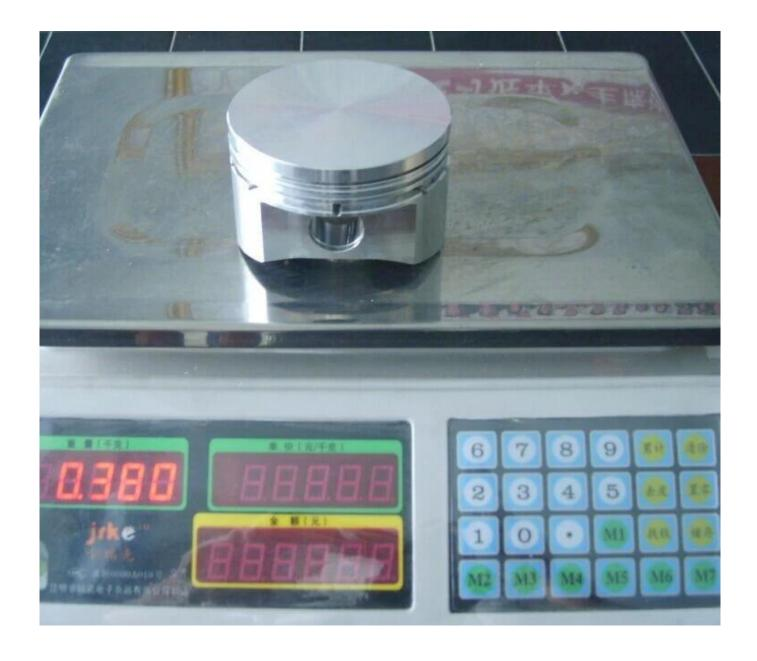
Note: The BMW forged piston are 380g per piece, light weight designed for high end application.
