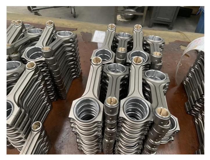
Forged Connecting Rods 144X22 VW & Audi RS3 are ready for packing. The rifle drilling application is available in all of hurricane 4340 steel connecting rods and they are sold separately, please contact us for more information if you are interested. And Audi RS3 X-beam rifle drilled connecting rods estimate weight is only 545 gram per piece.
