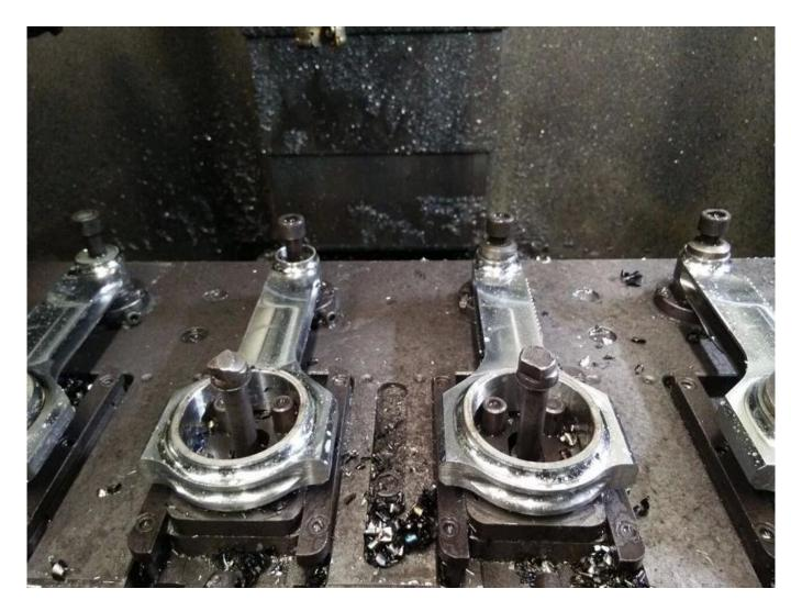
This is just one of the conrods progress we machined on CNC machine, to check more hurricane connecting rods production progress, please check directly at our news page: <u>Hurricane High Performance connecting rods - Process of machining rods</u> Or You can check our production video directly at Youtube Channel. please click the link: <u>VERSION 2 How it's made: 4340 forged connecting rod with CNC machine</u>
