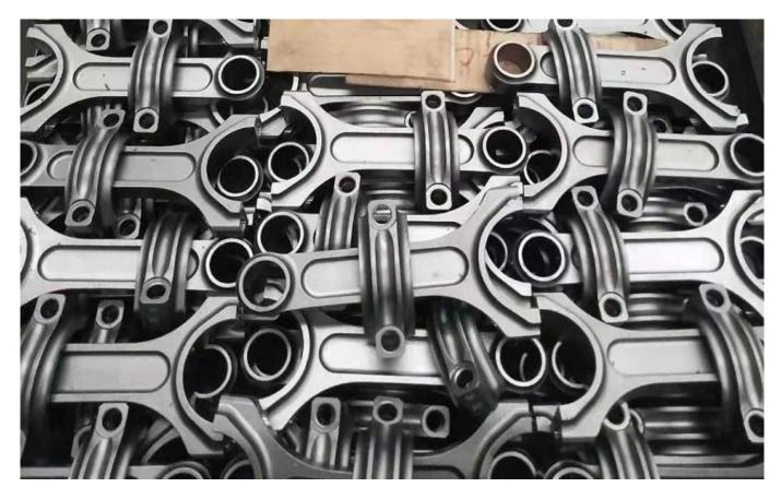
Note this is our production pictures for Renault 144x21mm I-Beam Connecting Rods.
