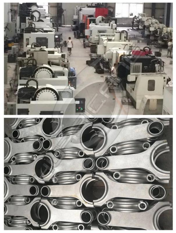
All big and small end bore honned with advanced honing machine for superior tight tolerance , per di mension inspected at workshop to guarantee high reliability .
