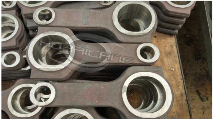
Per rod fully machine at Hurricane CNC center to handle maximum strength .
