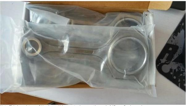
Note: This is a picture of Hurricane X-beam steel connecting rods 143mm Opel sample
