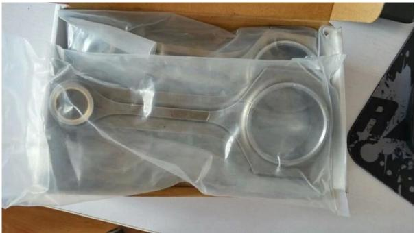
Note: This is a picture of Hurricane X-beam steel connecting rods 143mm Opel sample
