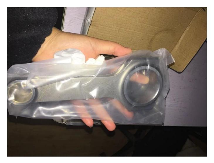
Mitsubishi 150mm length connecting rods for 4G63 engine is a hot item. Each set is balance weighted within +/-1g, Lighter and Stronger than OEM Mitsubishi Conrods, They are performance replacement connecting rod for all Mitsubishi EVO 4G63 models.
