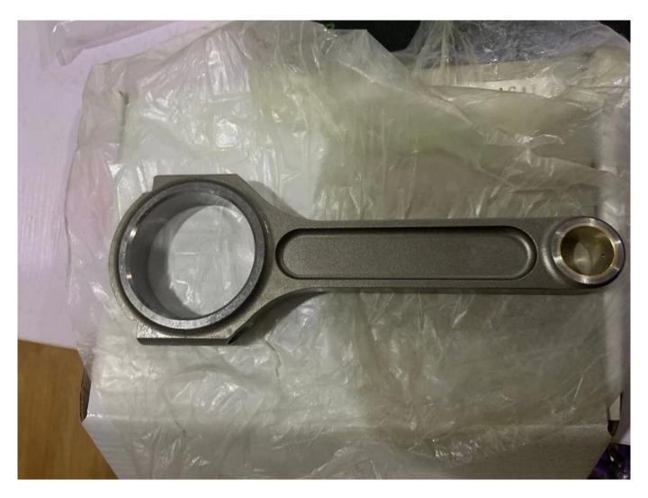
I beam Honda F23 Connecting Rods feature silicone bronze wrist pin bushes to ensure reliability.
