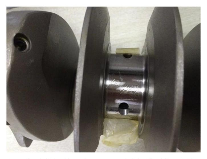
The Journal is required high precision Less than 0.01mm. Process by finish grinding, nitriding and polishing.
