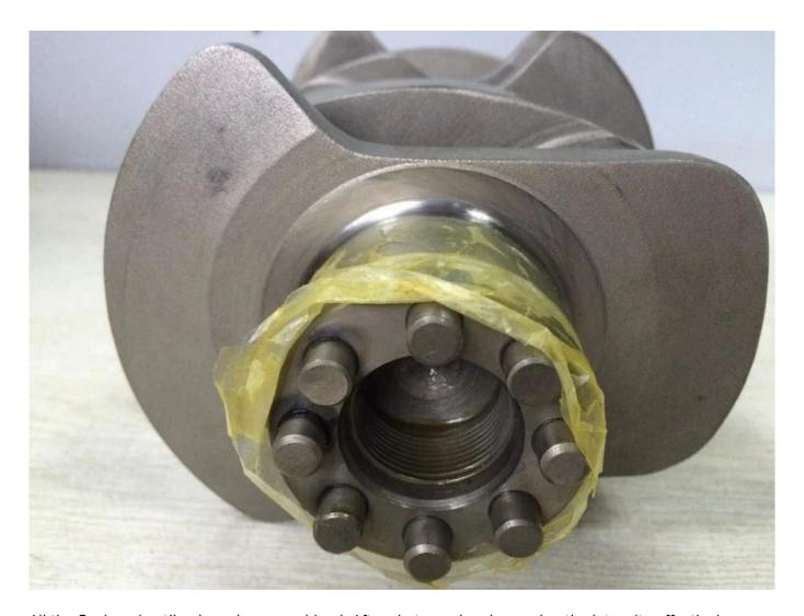
All the flank and outline have been machined. After shot peening, increasing the intensity effectively.
