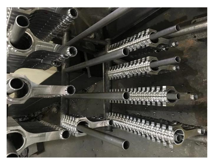
Forged Connecting Rods for Honda Civic CRX D16 D16A D16Y7 D16Y8 D16Z6 ZC are machined from ONE-Piece Forging, after Finishing maching surface and beam part, the Honda D16Z6/D16Y7 1.6Ltr 16V connecting rods will be polished and shot peened for improved fatigue life.
