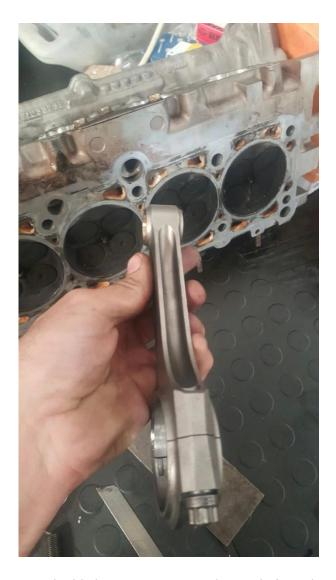
Noted: This is H-Beam Connecting Rods for Subaru EJ20 / EJ25 engines.
