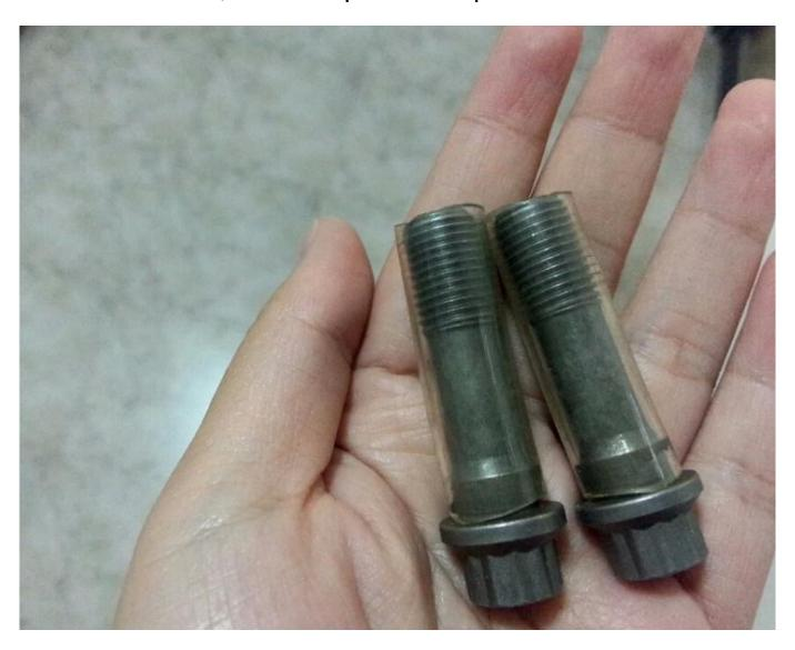
Hurricane performance 7/16 conrods cap screws, under head length 1.600" inch, weight 34 gram per piece.
