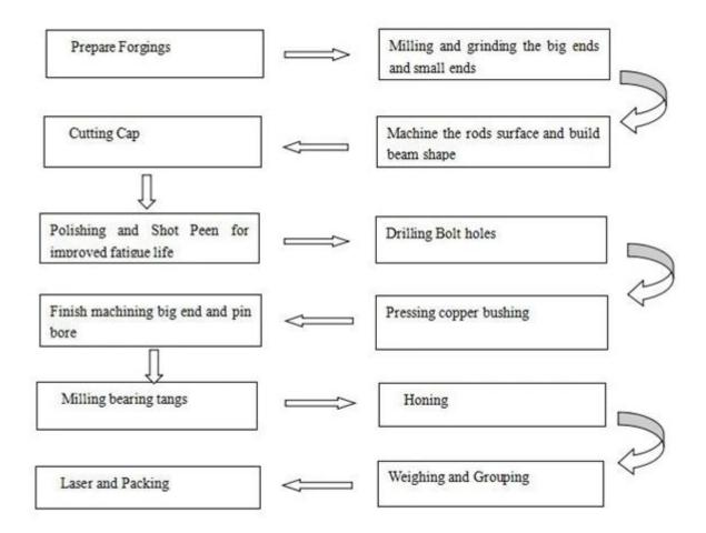
Hurricane can produce connecting rods based on used sample and detailed specs , if we OEM your style of connecting rods , here are some steps for your reference as below :
