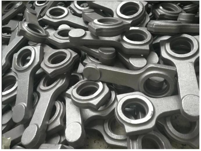
The forging process forces the grain into the shape of a connecting rod, resulting in a superior fatigue life.
