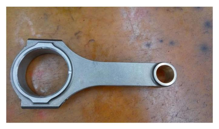
Note: Hurricane Toyota 2jzgte h beam connecting rods are designed for race engine application. drill a hole above the big end of the rod will reduce weight. big end design plus  $3 \times 45$  ° shoulder design will add more strength. The advise horsepower could reach 1000HP.
