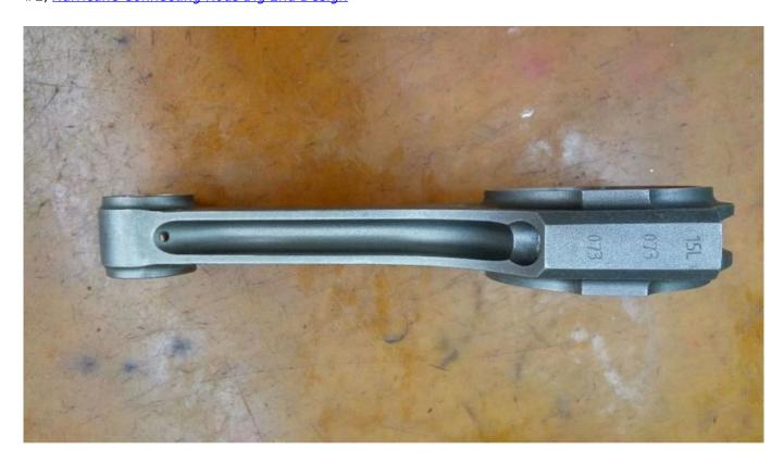
Note: toyota 2jz connecting rod Serial number are marked at shoulder part, specifically for re-uniting the rod and its cap after cutting.
