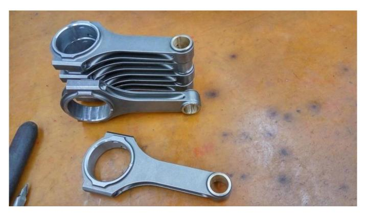
Note: Hurricane Toyota 2jz h beam conrods are packaged in set of 6, each set of 2jz conrods are balance weight to +/- 1g.
