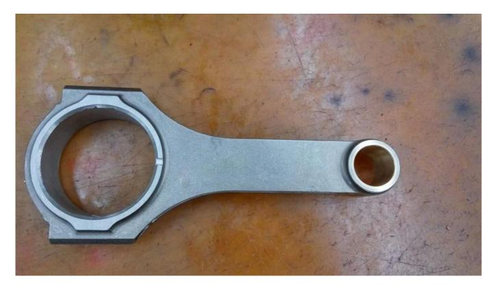
Note: Hurricane Toyota 2jzgte h beam connecting rods are designed for race engine application. drill a hole above the big end of the rod will reduce weight. big end design plus  $3 \times 45^{\circ}$  shoulder design will add more strength. The advise horsepower could reach 1000HP.
