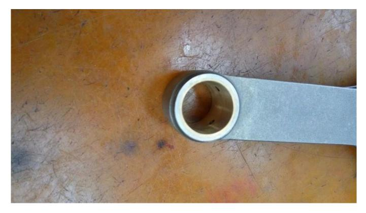
Note: Toyota 2jzgte h beam connecting rods Oil hole at Pin end providing lubrication.
