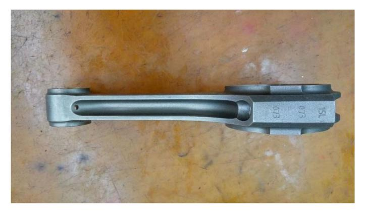
Note: toyota 2jz connecting rod Serial number are marked at shoulder part, specifically for re-uniting the rod and its cap after cutting.
