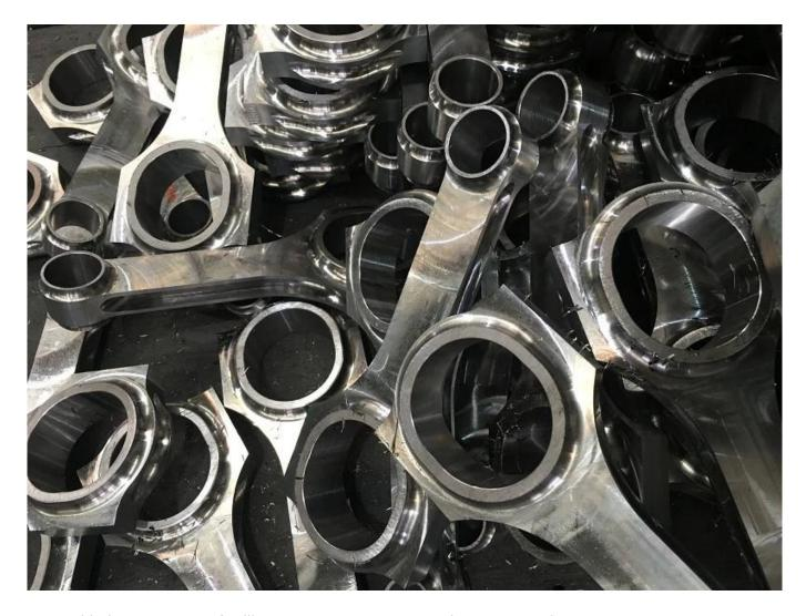
Note: This is a progress of mill MAZDA MIATA 1.6L/1.8L H beam connecting rods beam part and surface.
