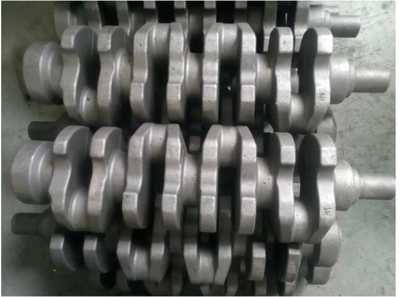
Remanufactured crankshaft for Ford 302 forgings: Multiple Die Stamp Forged From 4340 Chromoly (One Of The Strongest Materials Available For Crankshafts)
