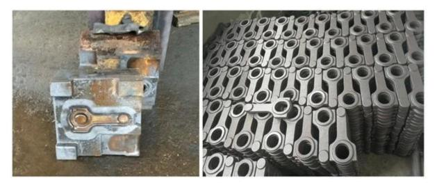
Then, machine rods on equipment from a forging to semi-finished to final rods
