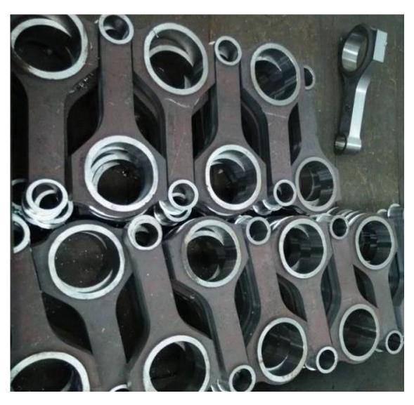
Note: This is a progress of drill Performance Replacement Forged Steel Connecting Rods for Buick engines big and small ends bore, which acts as a reliable locator in all process.
