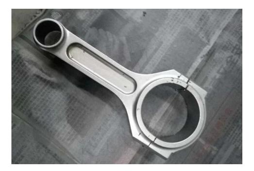
Note: This is a step of separate the beam from its cap. For more progress introduction please check: <u>Hurricane High Performance connecting rods</u> - <u>Process of machining rods</u>
