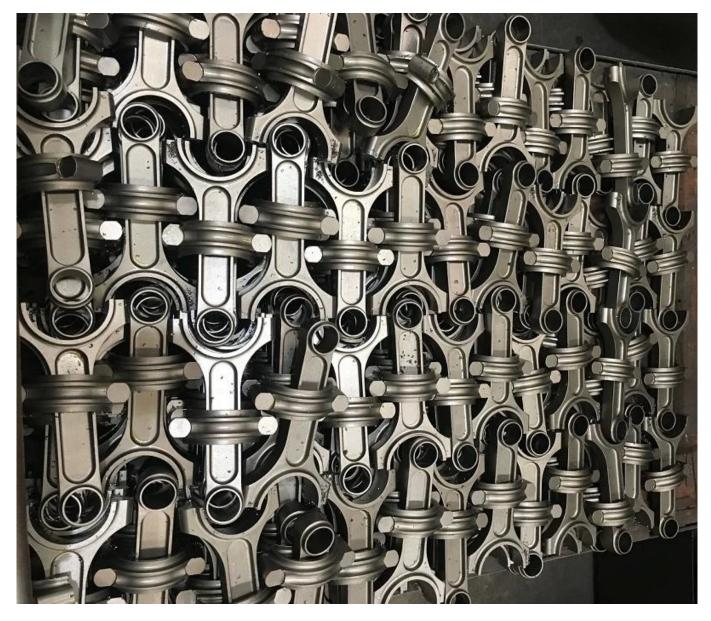
Note: The Toyota Celica, MR2 Turbo 2.0L 3SGTE 3S-GTE conrods will be polished (remove burrs and make surface smooth) and shot blasted first, then separate connecting rods from it's cap.
