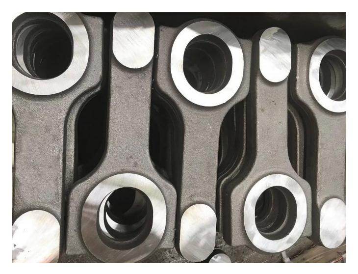
Note: This is our first machining operations, include face milling, grinding the big ends and small ends. You can check more detailed information at: <u>Hurricane High Performance connecting rods - Process of machining rods</u> Or check our opreations at Youtube Viedo: <u>How it's made: Connecting rod</u>
