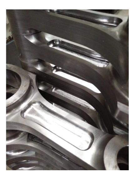
The duramax diesel connecting rods strong tapered I beam configuration can handle extreme engine loads. The tapered beam allows for some weight saving on the reciprocation end and gives increased clearance for fully boxed pistons.
