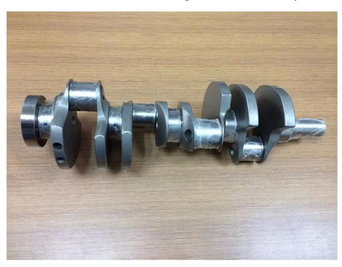
This is our finished Chevy LS1 Forged Crank 3.900" Stroke, It is designed for performance applications for off road, street and race applications. All GM LS1 4340 Forged Crank is CNC machined from One Piece of forged Chromoly steel, and they are micro polished and Nitrided. Nitriding is an expensive process where the crankshaft is exposed to gas under heat and pressure, this creates a really hard journal and added srength.
