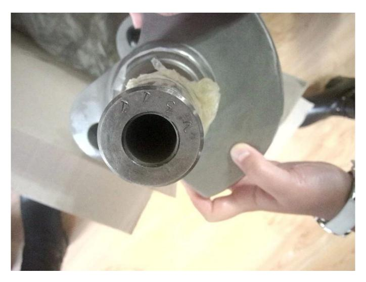
Hurricane finished LS1 Forged 4340 Steel Crankshaft 3.900" Stroke are also ground to EXACT sizes, magnafluxed, and dynamically balanced. much more every piece of our LS1 cranks have serial number (identify mark).
