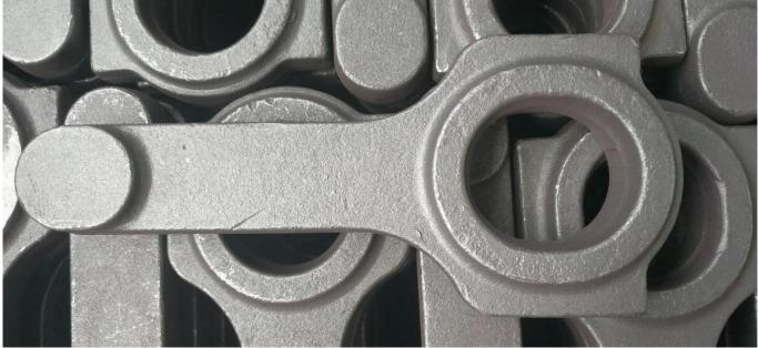
Note: forging 4340 steel, heat treatment: HRC34-38
