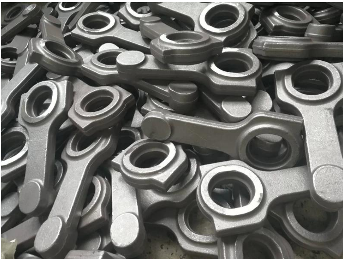
Featured product: HOLDEN L67 SUPERCHARGED 3.8L V6 - forged 4340 steel H-beam connecting rods
