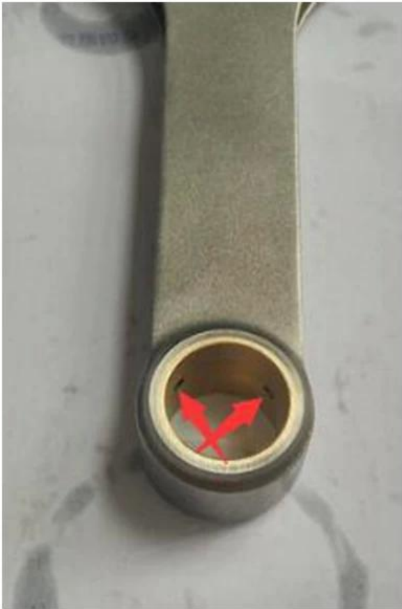
Two small oil holes drilled in the small end beam cut for well lubrication.
