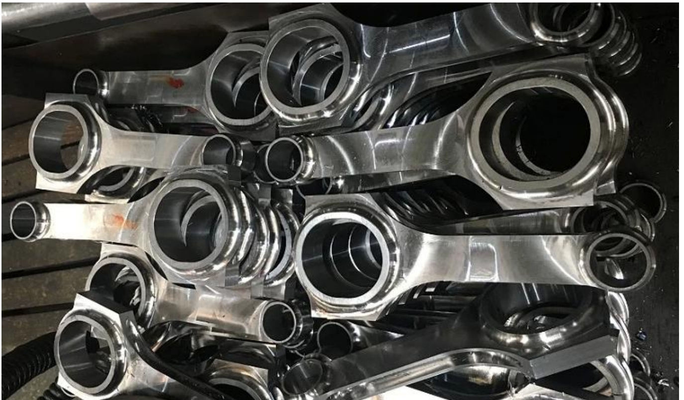
This is our H beam F20B connecting rods after CNC milled.
