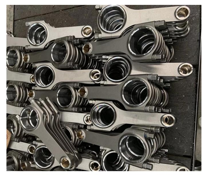
Those Honda F23 H beam Connecting rods are ready for Honning, mill bearing tags and packing. Fitti ng Info at below:
