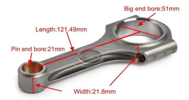
**Hurricane Speed and Performance** H-Beam connecting rods - Nissan RB26/RB25 are manufactured from **4340 steel forgings**, then They are fully machined, heat treated, stress relieved, shot peened, and magnafluxed, **all process of machining rods** post on website. Final all connecting rods Weight matched to +/- 1.5 grams. Perfectly round big and small ends. Bend and twist is tightly controlled. Cap fasteners are **3/8" ARP 2000 for the H-Beam and 3/8" ARP Custom Age 625+ for the H-Plus**.
