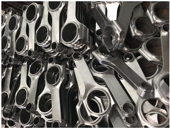
Note: H-Beam Connecting Rod for BMW E30 M3 S14 Polishing machine progress at Hurricane factory.
