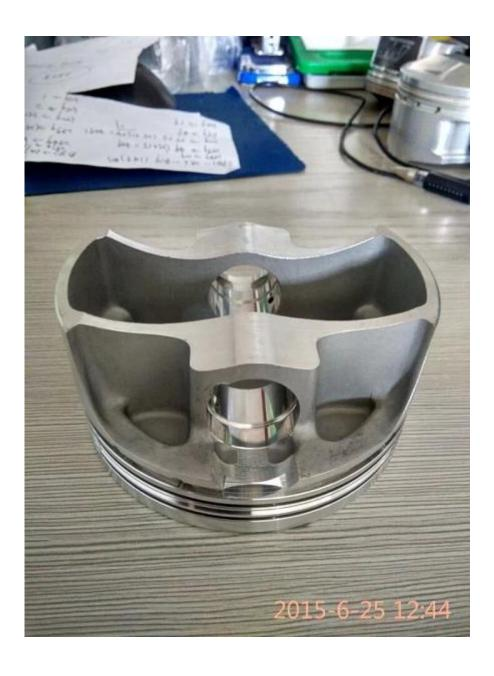
Note: Although The piston inner side is forging surface not finish machining, we still make it very smooth.
