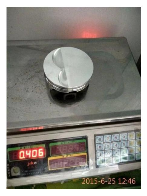
Note: high strength construction, but feature light weight to 406g per piece.
