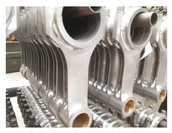
Note: Hurricane Connecting rod GM Duramax Diesel are all shot blasted and mico-polished. to view more of our conrods production process, please check:
