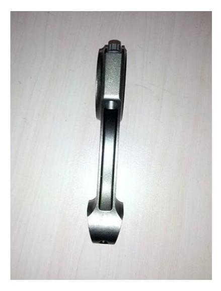
Note: GM Duramax performance connecting rods finished with tapered small  $\mbox{end}\ .$
