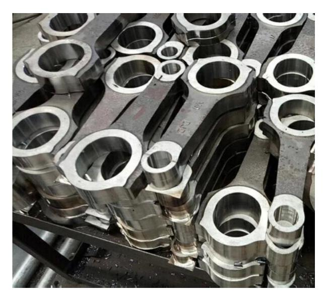
Note: This progress drill the big and small end bore, which acts as a reliable locator in all process.
