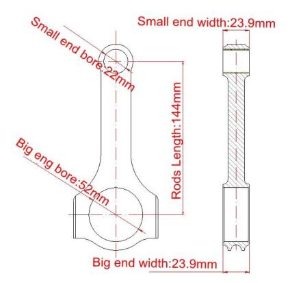
3. Bronze wrist pin bushings are fitted to each rod to increased wear resistance
