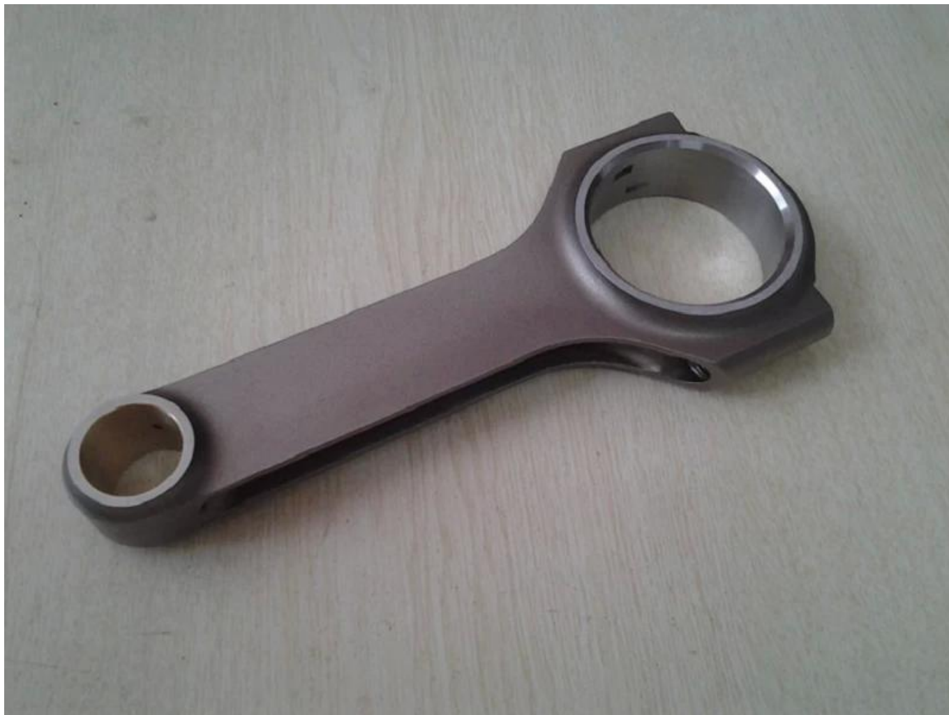
GM Chevy SBC Pro Sport H-Beam Connecting Rods, 5.850 length, 0.927 bushed fit wrist pin, 2.225 big end bore, Hurricane 7/16 rod bolts, Advertised Weight 550 grams, Set of 8
