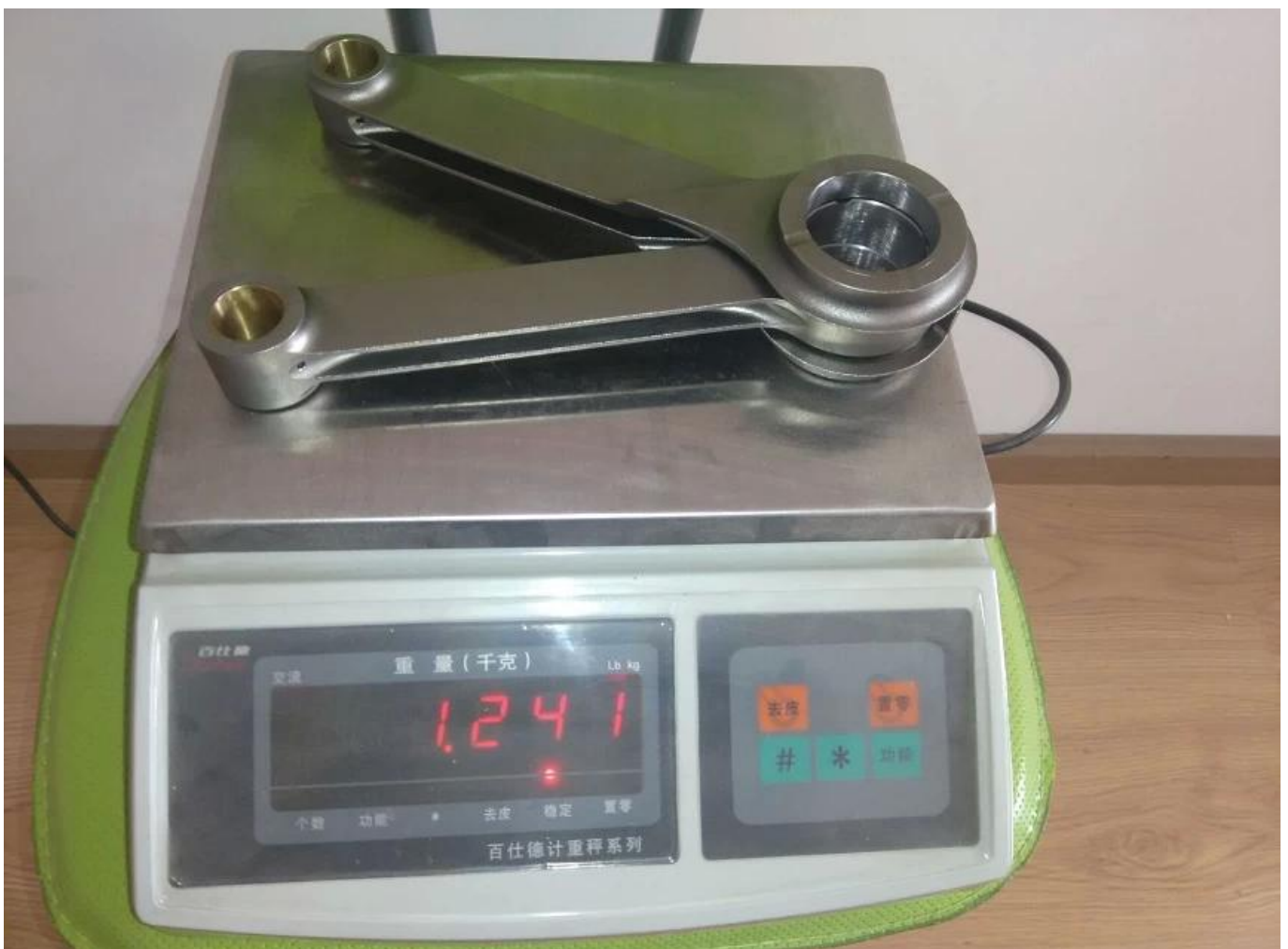
Hurricane 7.760" harley connecting rods weight is 1241kg per set.
