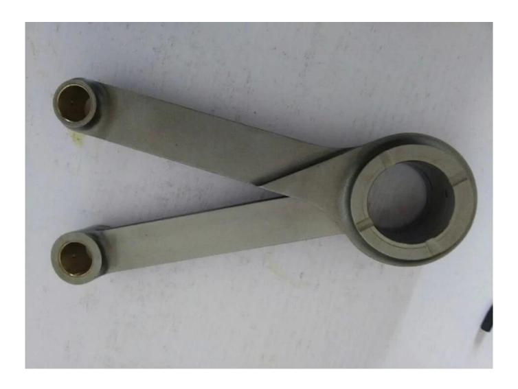
Those forged rods for Harley Davidson engine are made from 4340 steel forgings and finished on Computer numerical control production line. they appearence is very smooth, hard to see tool vestige. All hurricane connecting rods are shot blased and polished, will increase connecting rods strength, toughness and resistance to impact.
