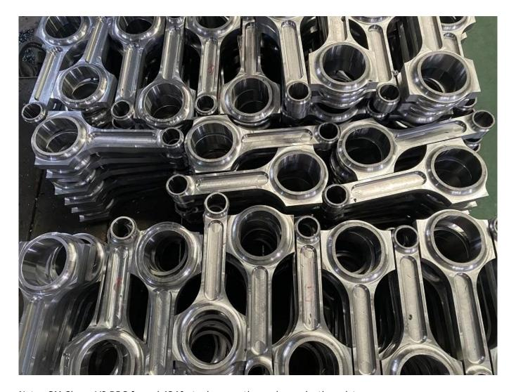
Note: GM Chevy V8 BBC forged 4340 steel connecting rods production picture.
