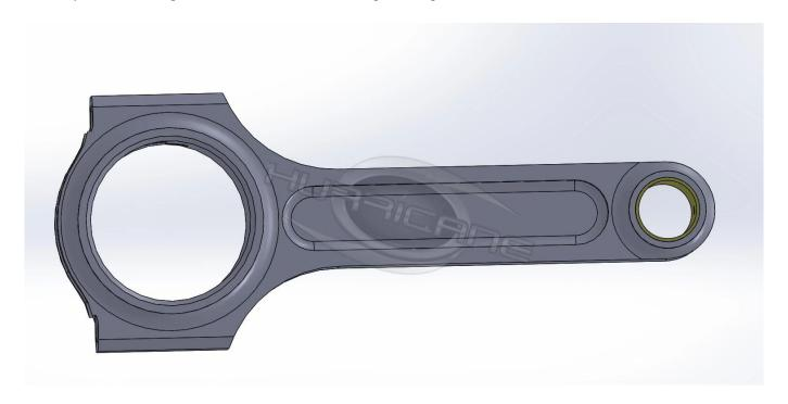
Per rod is heat-treated with temperature  $860^{\circ}\text{C} \sim 880^{\circ}\text{C}$ , the HRC rate 34-38. Per rod had been magnafluxed and demagnetized , and fully shot-peened to finish the surface well . Per sets weight matched within 2gram, and fully removed burrs before shipment .
