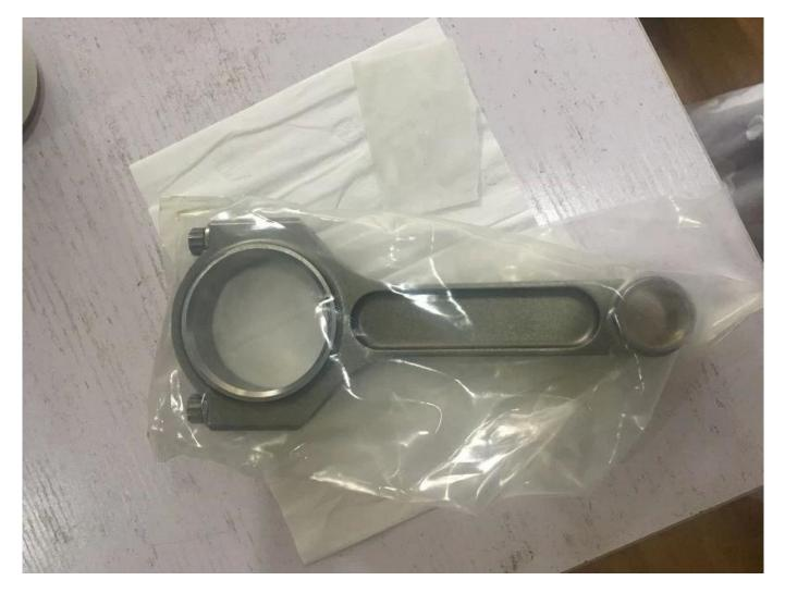
Racing rod for Ford 460 6.605" I-beam are the strongest, advise horsepower 1600HP.
