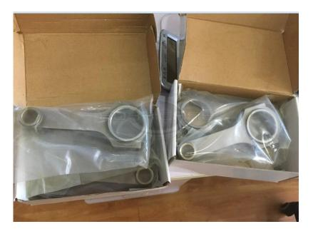
Hurricane new finish honda h22 5.636" H beam connecting rods installed with <u>Hurricane replacement 3/8 rod bolts</u>. Currently we can not offer Original ARP2000 bolts, but if we have cooperation, you can ship original ARP bolts to Hurricane factory for free install.
