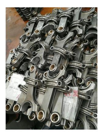
Each rods are finish-honed by SUNNEN equipment with high tolerance standrad at <a href="https://hurricane"><u>Hurricane</u></a>
