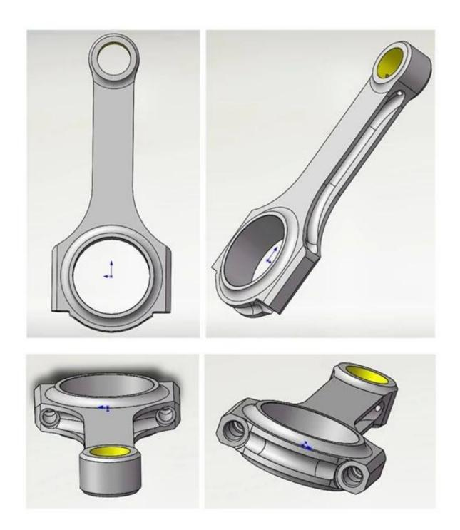
Each rod is multi-stage heat-treated, <u>100 percent machined</u>, and then shot-peened to stress-relieve the metal. The rods have precision cap alignment sleeves to positively locate each rod cap, silicon bronze bushings for floating pin models—and are available in stroker models that allow additional cam-to-rod clearance for large stroke combinations.
