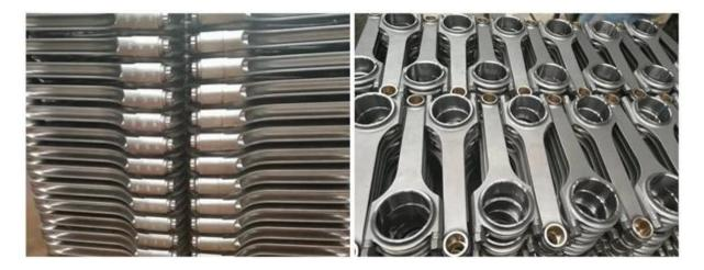
They come standard with 190,000 psi rated **ARP 8740** and 230,000 psi rated **ARP 2000** rod bolts, or 265,000 psi rated **ARP L-19** bolts as upgrades. Instructions and rod bolt lubrication are included.
